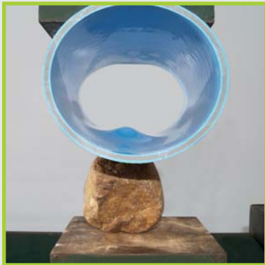
Toughness of the pipes demonstrated by point loading the pipe with a rock
